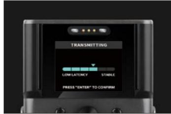
The B-8 and B-6 Pro offer 6 Stability Levels, while the B-7 Pro provides 3.
