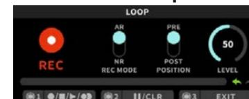
The AAS also includes a 30 second stereo phrase looper. This powerful little looper can be used in either Auto Record or Normal Record modes. Additionally, it can be set to the pre or post position in the signal path.
