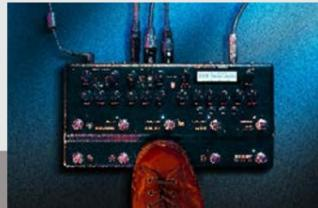
The knob layout, toggle switches, and foot switches of the TRIDENT are akin to stomp boxes, you can engage /disengage the effects freely. The SELECT & PARAM encoders with LCD display deliver more parameter details, block order / status.
