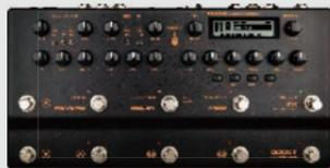
The TRIDENT uses a one-piece die-cast aluminum chassis. It's solid, strong, and built for live performance.
