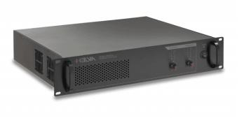
Helvia paid high attention to safety, reliability and duration over time of these amplifiers. Each channel is equipped with muting system at power on, signal limiter, thermal protection and current limitation. The cooling system with fan speed controlled by internal temperature, is also reinforced thanks to the 19" 2U Rack standard size that increases the thermal dissipation.
