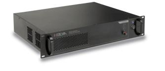
Helvia paid high attention to safety, reliability and duration over time of these amplifiers. Each channel is equipped with muting system at power on, signal limiter, thermal protection and current limitation. The cooling system with fan speed controlled by internal temperature, is also reinforced thanks to the 19" 2U Rack standard size that increases the thermal dissipation.
