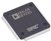
At the core of this system's audio processing capabilities is a powerful digital signal processing (DSP) engine built around SHARC-based processors from Analog Devices. These DSP chips deliver high performance with speeds up to hundreds of millions of instructions per second, supporting both 32-bit and 40-bit floating-point computation for incredibly accurate and detailed audio calculations — ideal for professional-grade sound processing tasks.
