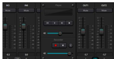
The SoniX MD features a convenient front-panel USB port, enabling real-time audio playback from, and recording to, external USB drives. Both playback and recording are fully integrated into the matrix, allowing them to function as additional stereo sound sources and stereo outputs. Like all other analog and Dante™ inputs and outputs, these USB sources can be freely configured to suit any setup, providing maximum flexibility in routing and audio management.
