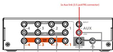
Connect multiple GM44L units via 3.5 mm stereo jacks to **expand the number of zones** with no need for DSPs or complex digital matrices. A scalable solution for those who want to start small and grow the system over time.
