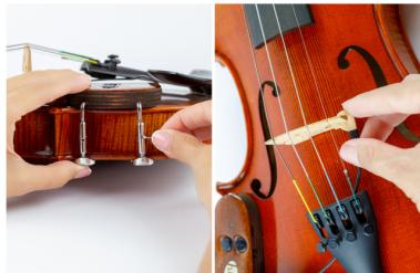
Mount the pickup jack housing on the lower bout, just below the waist on the 4th (G) string side of your instrument. Adjust the height of the barrel clamps to tighten the pickup to the instrument.
