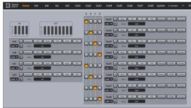
The control software is extremely sophisticated but equally simple and intuitive. Each input and output are represented by a real path that the signal follows within the SoniX 4800F. Pressing each of the buttons takes you to the relevant screen that allows the modification of many parameters.
