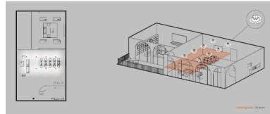
Thanks to the integrated transformer for **100V/70V** lines, this high-impedance loudspeaker **allows several speakers to be connected in parallel over long distances without significant loss of power or audio quality**, making it ideal for distributed systems in hotels, shopping centres, schools or public facilities.
