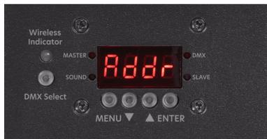
If for aesthetic or distance issues the normal DMX cable connection is not for you, no problem. Portrait Q-Air fixtures can be controlled **up to 300m** without cables thanks to **2.5GHz Wireless DMX**, which operates in the license-free ISM band from 2.400 to 2.525 GHz and adopts the highly efficient **GFSK modulation system**. This protocol provides **7 IDs, each with 512 DMX channels**, and is a fast and safe solution even in rather complex projects.
